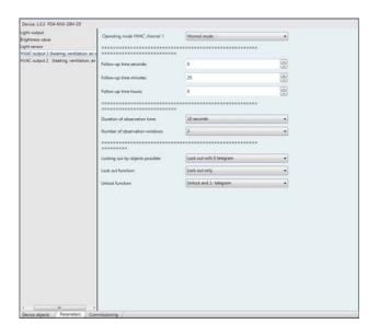
The HVAC channel (Heating Ventilation and Air Conditioning) has been designed so that systems with high energy consumption can be started with a time delay. In addition, an alarm indicator can be simulated with an HVAC channel.
