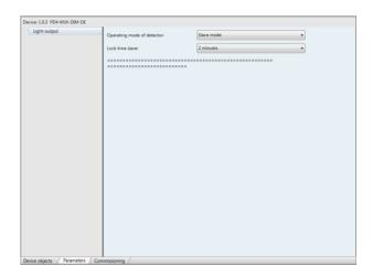
The locking time is the only parameter that can be set in slave mode. It specifies the dead time between sending two signals.
