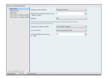
Permanent dimmer mode is used in areas where a specific lux value should be provided at all times (bank lobby, passage, etc.).
