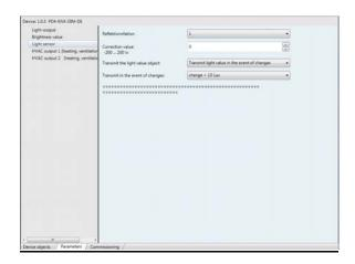
B.E.G. KNX occupancy detector offers the option of outputting the measured light value in the room to the BUS via a 2-byte object.
