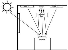
To make this adjustment, a lux meter must be positioned at the point where the desired lux value is to be achieved. The lighting must be switched on (please allow 10 minutes for fluorescent lights to warm up). The lux value is then measured, e.g. on the desk. Finally, the light value on the ceiling should be determined. To do this, a lux meter can be held at the position of the occupancy detector or the occupancy detector or the occupancy detector can output the lux value on the BUS.
